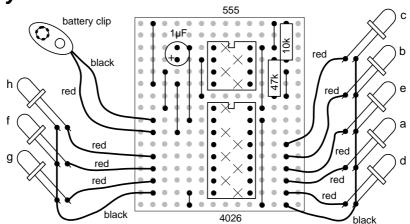
11 tracks to cut under the chip holders, shown  $\times$  Note: do NOT cut between pins 2 and 15 of 4026.
